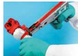
Tighten cable ties
