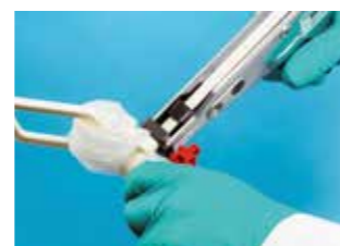
Tighten cable ties
