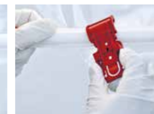
Loosen safety lock by turning it slightly
