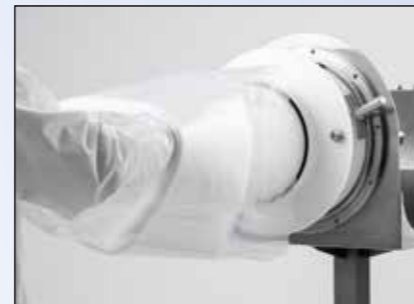
Put on the Continuous Liner
