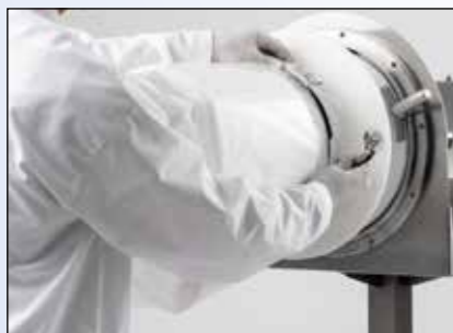
Seal the Continuous Liner on the carrier tube
