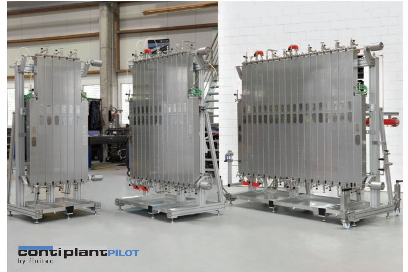
ContiplantPILOT reaction system made from Hastelloy C-22, including sampling valves, bursting discs and pressure and temperature sensors
