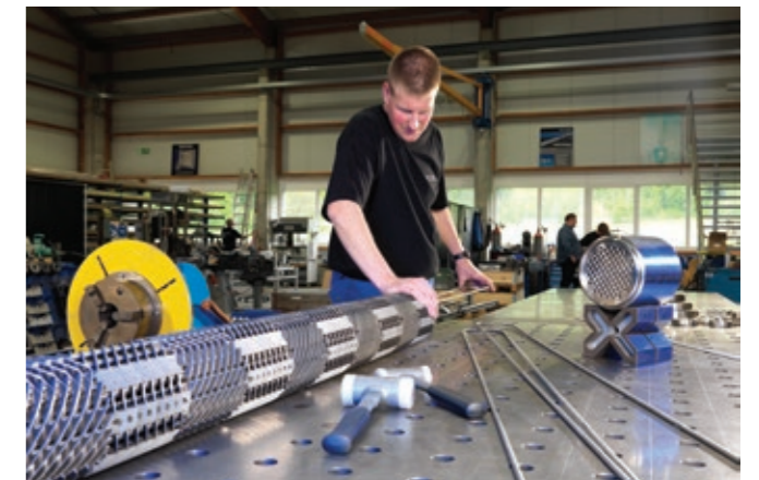
Structure of a Fluitec CSE-XR mixer / heat exchanger
