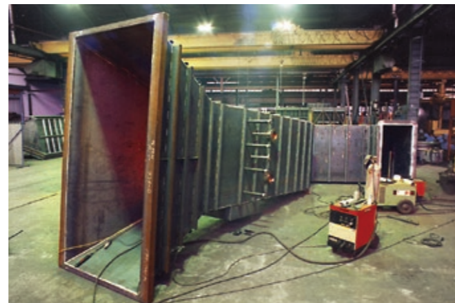
Flue gas duct for a DeNOx system
