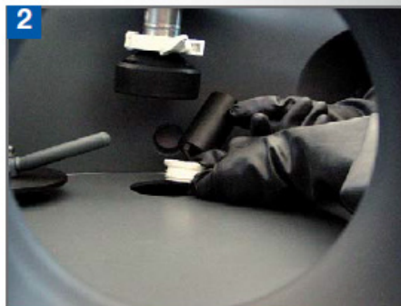
2 Opening of the drum by removing the screw cap with a specially designed tool
