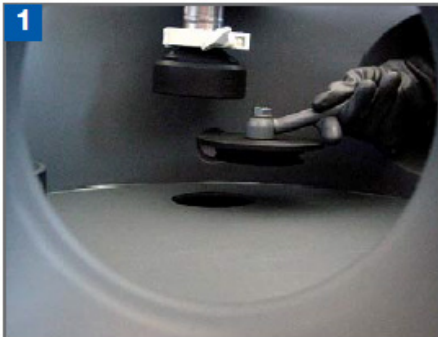
1 Access to the drum inside the DCS by removing the protection cover
